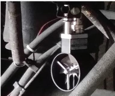
Over-the-road data acquired from anemometers and thermal sensors show trailer skirts reduce air flow and increase average brake temperatures 41%.
